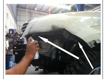
4. Spray paint the metal underside of the fender and the underside of the headlamp black.
