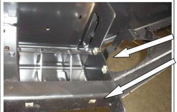
21. Fit cage nuts and nylon plugs to the bull-bar.
