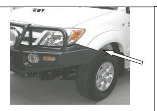
40. Adjust the bull bar position up/down and in/out to achieve uniform gaps between the bar and the fenders on each side of the vehicle. The nominal clearance between the bull-bar and the fenders is 20mm. Tighten the bolts fitted at steps 37 & 40 to specified torque.
