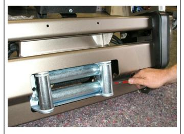
33. Fit roller fairlead into cutout and refit bolts and tighten firmly.
