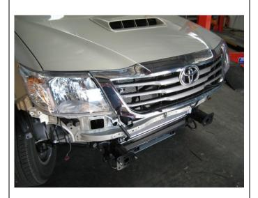
7. Reassemble the vehicle's grill removed at step 1; make sure the 2 lower grill tabs are pushed into the clips in the lower grill bracket. Bend lower grill bracket tab upwards slightly.
