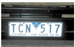
55. Fit the plastic plugs into the square holes in the lower or upper pan depending on fitment. Fit the number plate to the bull bar using the black self-tapping screws.
