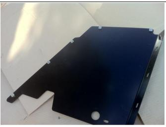
46. Fit the M6 cage nuts to the wing stone guards as shown.
