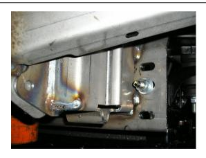
39. Position the bar on the vehicle and fasten it to the chassis studs using the M10 washers, spring washers and nuts provided. Once satisfied that the bar is centrally positioned on the vehicle properly tighten the M10x 1.25P nuts.
