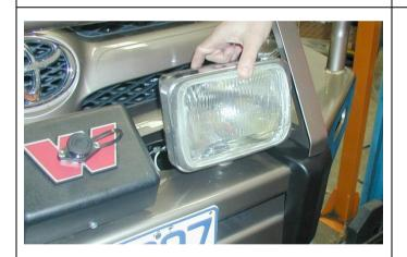
54. If fitting optional driving lights to vehicle do so at this stage. Guide ratchet spanner between the upper and lower pans, as shown, to tighten the lights to the bar.
